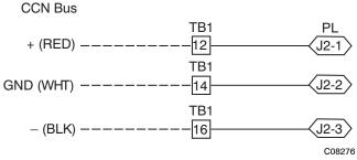
Fig. 58 - PremierLink CCN Bus Connections
